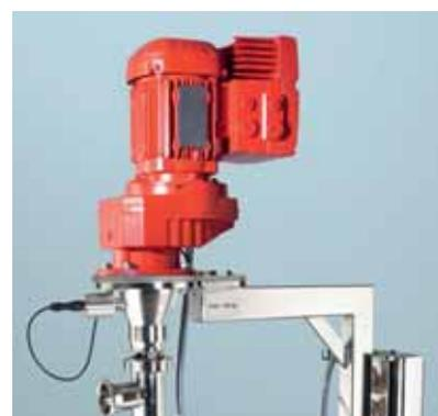
The bearing flange with impulse generator enables an indirect volume measurement.
