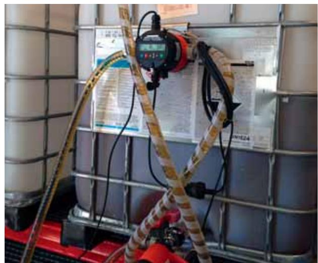
Semi-automatic filling with FMC 100 and switching amplifier FSV 100 from IBC.
