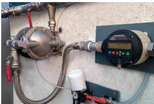
FMC 100 in combination with air-operated diaphragm pump for manual use.
